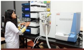
Tandem LC with ion trap mass analyzer (LC-MS)
